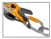
The Am'D carabiner has an asymmetrical D shape that is ideal for attaching equipment such as descenders or positioning lanyards. Use of the CAPTIV positioning bar favors loading of the carabiner along the major axis, limits its flipping and keeps it attached to the device or lanyard.
